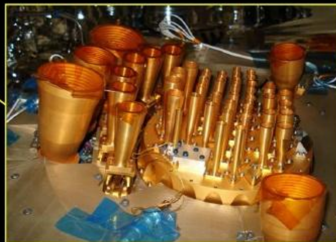
LFI Radiometers 30-70 GHz, T = 20 \text{ K}
