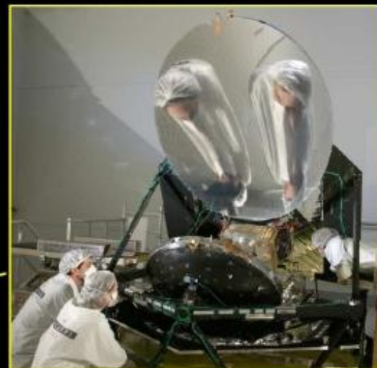
Planck Telescope 1.5x1.9m off-axis Gregorian T = 50 \text{ K}
