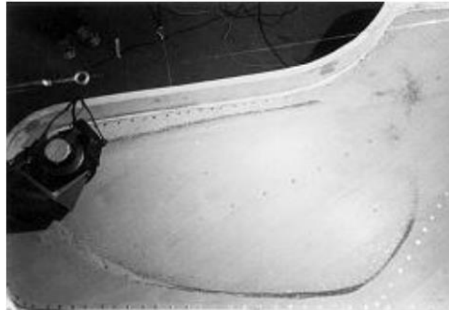
Fig. 17. First (lowest) soundboard mode at 49 Hz.
